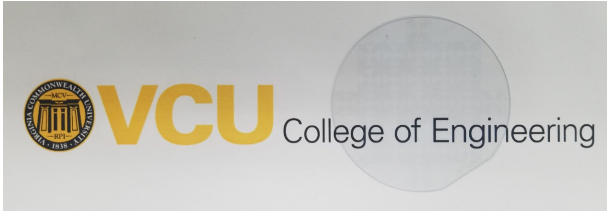
Figure 52 Fabricated GZO band pass filter with Virginia Commonwealth University College of Engineering Logo for background.
